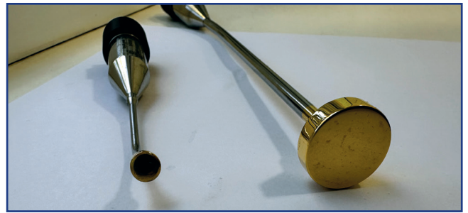
Figure 2 – Probes with a diameter of 5 and 20 mm
